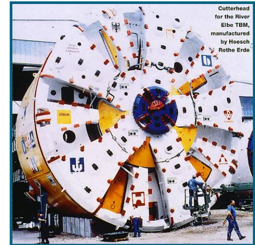
Elbe Tunnel Slurry Machine
